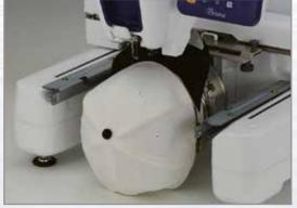
Set cap directly onto the machine
