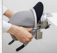
Sliding and ratchet frame fixing
